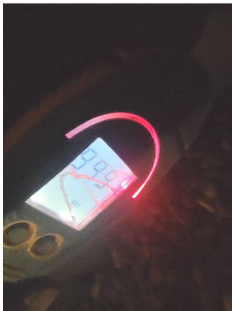
Moisture Meter Showing Wet
