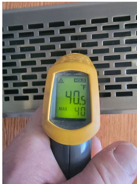
Supply Temperature Drop Excessive
